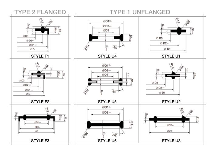
SICHEM<sup>®</sup> seals offer the best technical solution far all TRI-CLAMP standards, the most common connection in the pharmaceutical and food processing industries. Produced with modified and restructured ptfe, SICHEM<sup>®</sup> seals show excellent mechanical properties: no extrusion and no cold flow and a high resistance to almost all chemicals. This allow SICHEM<sup>®</sup> seals to be safely used in all the cleaning and sterilizing processes.
